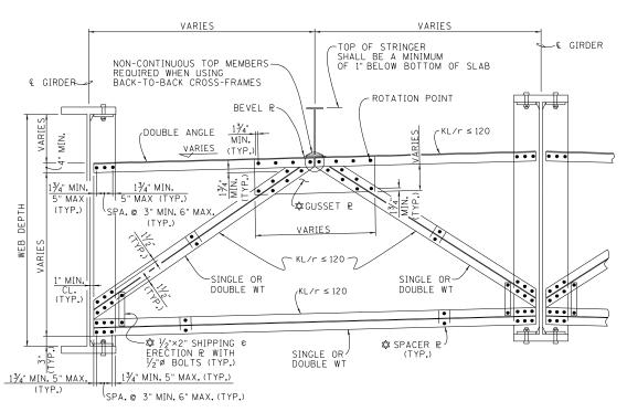
TYPICAL K-FRAME WITH STRINGER (☆PLATE THICKNESS SHALL MATCH STIFFENER THICKNESS WHEN USING DOUBLE MEMBERS AND NUMBER OF SPACER PLATES REQUIRED SHALL BE DETERMINED BY DESIGN.) ORIENTATION OF K-FRAME WITH STRINGER SHALL BE AS SHOWN.
