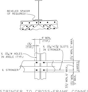
STRINGER TO CROSS-FRAME CONNECTION (NOTE: 1"Ø ASTM F3125 GRADE A325 BOLTS TO BE USED.) (TYPICAL ALL LOCATIONS)
